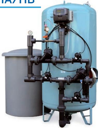
The tank is made of steel and it is protected internally by a food-grade layer of epoxy resins of controlled thickness and covered externally by a layer of enamel paint. The harness is in corrosion-proof PVC Noryl. Ultra Line HA softeners are available in tanks ranging from 500- to 1200-mm in diameter. For tanks with 950- to 1400-mm diameter it is available also a HB version, with larger harness, in order to facilitate higher service flow rates.
