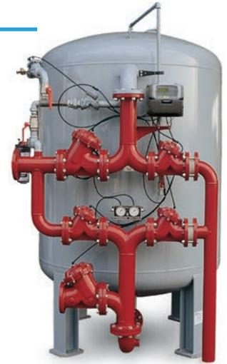
The tank is made of steel and it is protected internally by a food-grade layer of epoxy resins of controlled thickness and covered externally by a layer of enamel paint. The cycles are controlled by diaphragm valves, made of epoxy painted cast-iron. Ultra Line HB softeners are available in tanks ranging from 1500- to 2500-mm in diameter.
