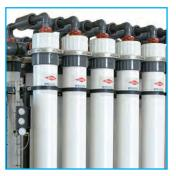
With a nominal pore diameter of  $0.03~\mu m$  the UF technology efficiently removes pathogenic agents, most viruses and bacteria. Additionally the high porosity membranes, compared to the standard capillary ones, allow a high flow rate at the same supply pressure of the membrane.
