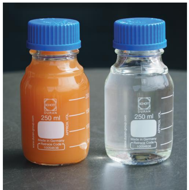
Spoelwater vóór en na de zuivering Backwash water before and after purification
